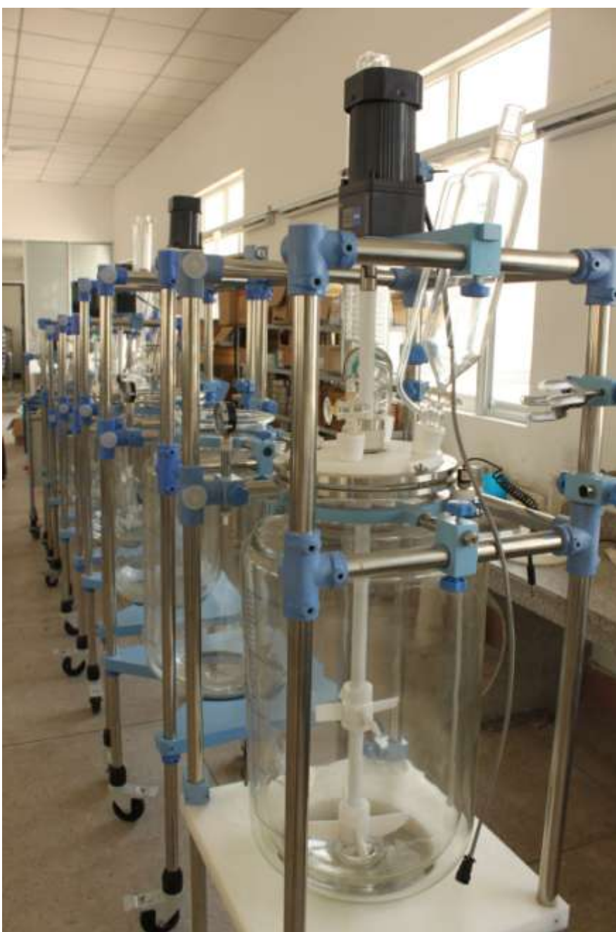
Pilot Scale Jacketed Glass Reactor
